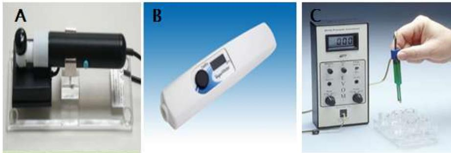
Fig. 2. The picture of Tewameter(A), Vapometer(B) and Electrical resistance system(C)
